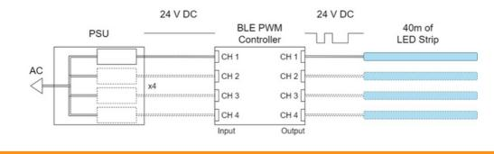
The BLE mesh network facilitates energy reduction by incorporating occupancy sensor control. The system uses Passive Infrared (PIR) sensors to detect motion, within the corridors, that trigger the PWM controllers, via the BLE mesh, to control the luminaires` light output. Further reasons why the BLE mesh is well-suited for this application is as follows:
